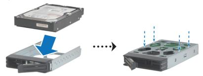
• For 2.5" Hard Disk: Place the hard disk in the hard drive tray, turn the tray upside down, and then tighten the screws to secure the hard disk.
