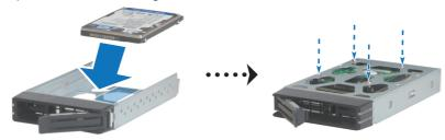
3 Insert the loaded hard drive tray into the empty hard drive bay.
