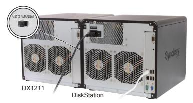
If the AUTO/MANUAL switch is set to MANUAL, press the POWER button to turn on RX1211/RX1211RP.
